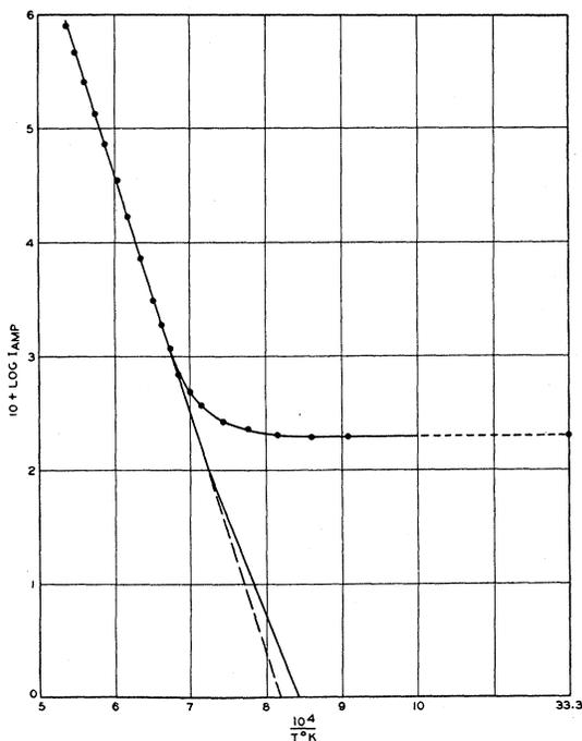
FIG. 7. Electron emission from molybdenum at  $F=1.05 \times 10^6$  volts/cm. The intersecting straight lines give the thermionic emission.
