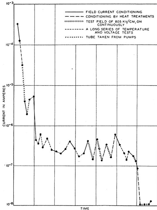
FIG. 5. Early life history of a molybdenum filament. A test field of 805 kilovolts/cm was used. The time extended over about 20 days.
