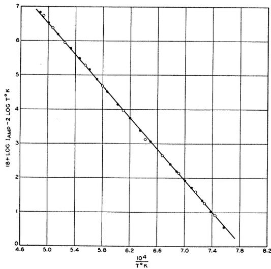
FIG. 2. Richardson plot of thermionic emission from tungsten.  $F=1.2 \times 10^4$  volts/cm. Dotted circles for decreasing temperatures; open circles for increasing temperatures.
