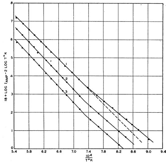
FIG. 6. Richardson plot of thermionic emission from molybdenum. Curve 1,  $F=4.4 \times 10^5$  volts/cm; curve 2,  $F=1.0 \times 10^4$  volts/cm; curve 3,  $F=1.0 \times 10^3$  volts/cm. Add 0.6 to ordinate.
