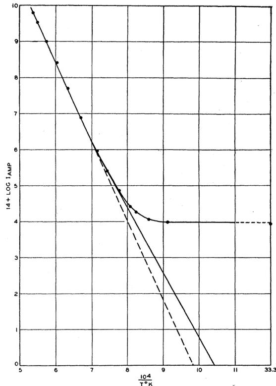
FIG. 8. Electron emission from molybdenum at  $F=8.13 \times 10^6$  volts/cm. The intersecting straight lines give the thermionic emission.
