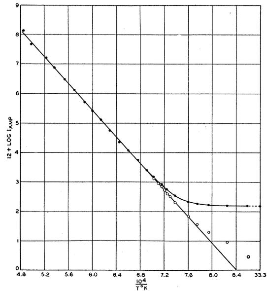
FIG. 4. Electron emission from tungsten at  $F=5.42 \times 10^5$  volts/cm. Dotted circles are experimental points; open circles show the difference between measured currents and current at  $300^\circ\text{K}$ .
