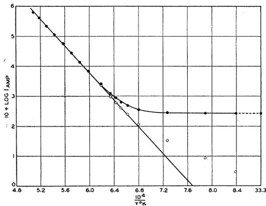
FIG. 3. Electron emission from tungsten at  $F=9.47 \times 10^5$  volts/cm. Dotted circles are experimental points; open circles show the difference between measured currents and current at  $300^\circ\text{K}$ .
