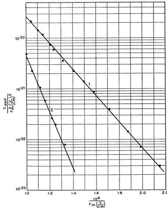
FIG. 9. Electron field currents from pure tungsten and molybdenum. Curve 1, tungsten; curve 2, molybdenum.
