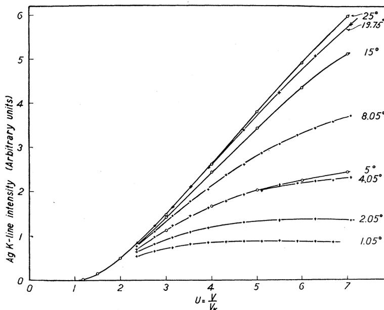
FIG. 1. Ag line intensities for constant current.
