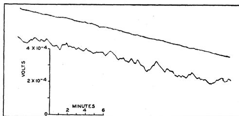
FIG. 5. Record showing fluctuations with resistance in circuit.
