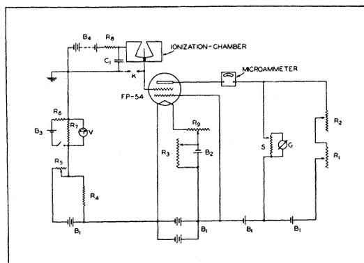
FIG. 1. Single-tube circuit used by DuBridge.
