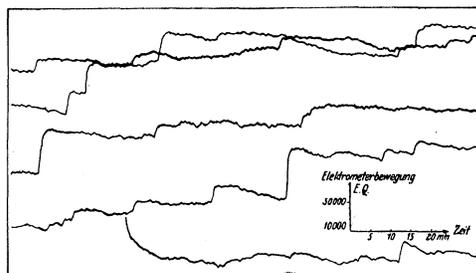
FIG. 7. Specimen record by duant electrometer (after Pose).
