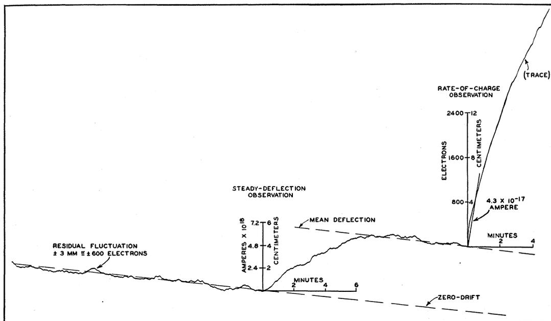
FIG. 6. Record showing deflection due to small steady current.
