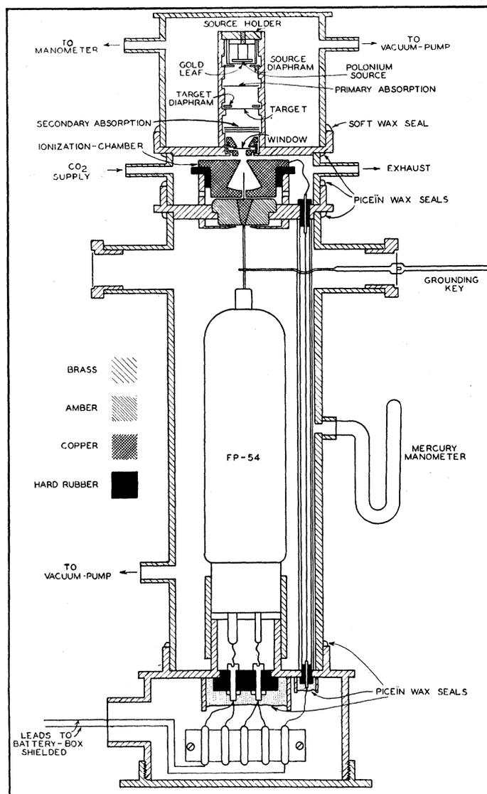
FIG. 2. Ionization-chamber and electrometer-mounting.
