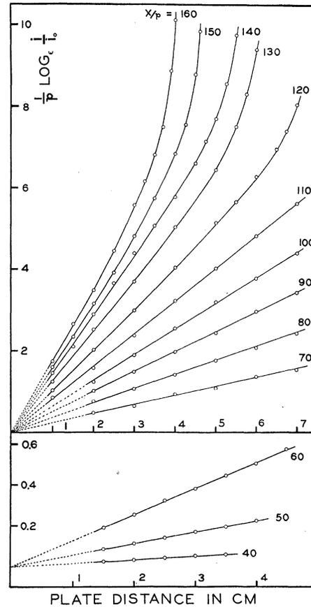
FIG. 1. Current as a function of plate distance.
