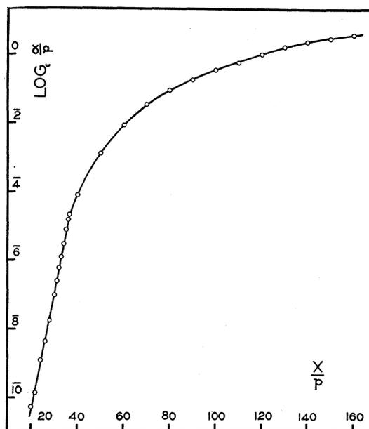
FIG. 3. Logarithm of  $\alpha/p$  as a function of  $X/p$ .
