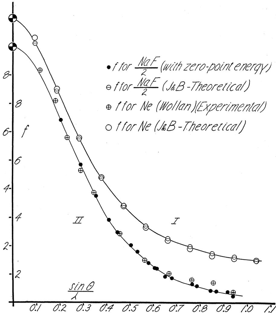
FIG. 3. Curve I, theoretical  $f(NaF)$ ; curve II, experimental  $f(NaF)$  with zero-point energy, shifted one unit in the negative direction of the structure factor axis.
