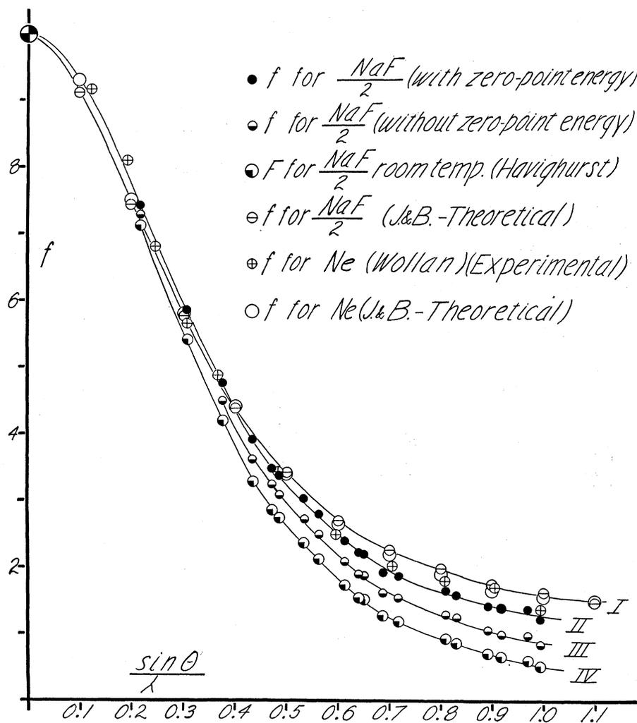
FIG. 2. Curve I, theoretical  $f(\text{NaF})$ ; curve II, experimental  $f(\text{NaF})$  with zero-point energy; curve III,  $f(\text{NaF})$  without zero-point energy; curve IV,  $F(\text{NaF})$  room temperature.
