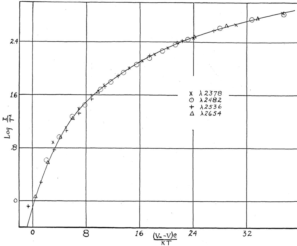
FIG. 8. Analysis of current-voltage curves for Mo.
