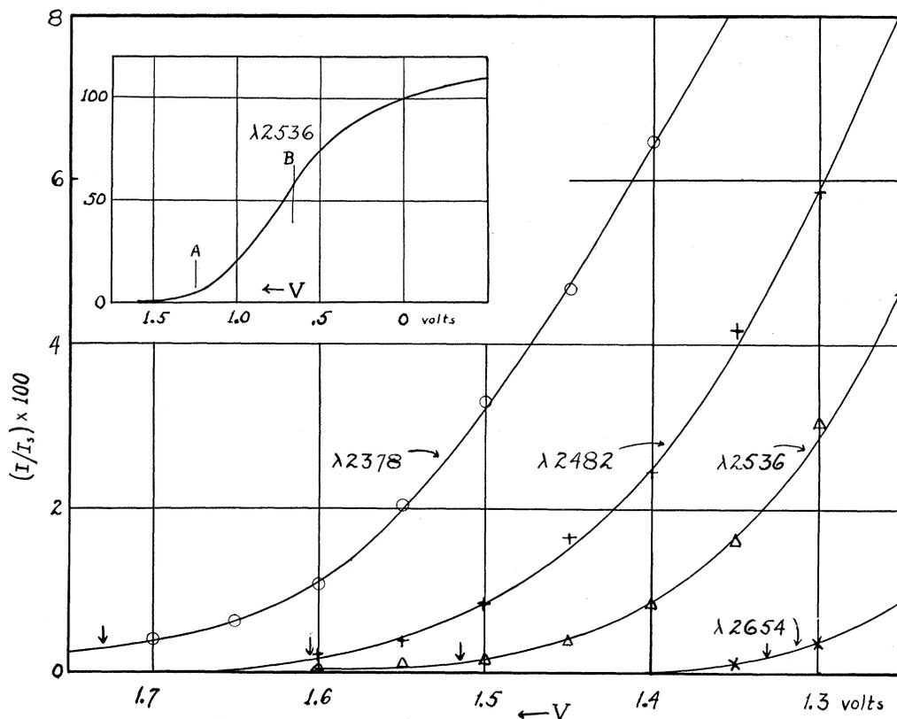
FIG. 7. Experimental current-voltage curves for Mo at room temperature, using parallel plate electrodes. Inset, complete curve for  $\lambda 2536$ . Lower curves, magnified portion of the tail.  $I_s$ =saturation current. Arrows indicate values of  $V_m$  for  $0^\circ\text{K}$ .
