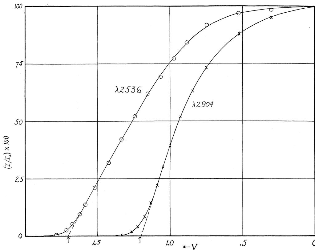
FIG. 12. Observed current-voltage curves for clean Mo. Broken lines indicate approximately the theoretical shape of the tail for  $0^\circ\text{K}$ . To avoid congestion only a few of the observed points are plotted.
