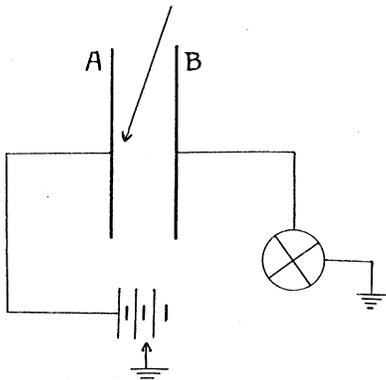
FIG. 2. Parallel plate method.
