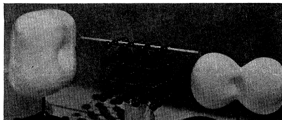
FIG. 6. On the left, E_\theta for an iron crystal elastically stretched 1 percent along a [100] axis. On the right, E_\theta for an iron crystal elastically compressed 1 percent along a [100] axis.
