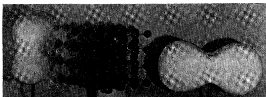
FIG. 7. On the left, E_\theta for an iron crystal elastically stretched 1 percent along a [110] axis. On the right, E_\theta for an iron crystal elastically compressed 1 percent along a [110] axis.
