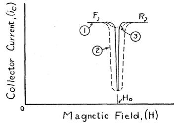
FIG. 4. Variation of collector current near resonance.
