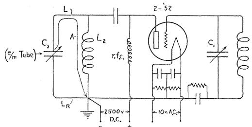
FIG. 5. Oscillator for supplying the radiofrequency voltage.
