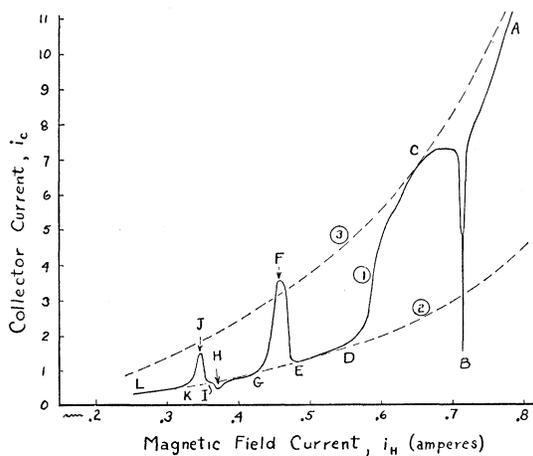
FIG. 7. Variation of collector current with magnetic field at a frequency of  $3.7920 \times 10^7$  cycles and a peak voltage of 2400 volts.
