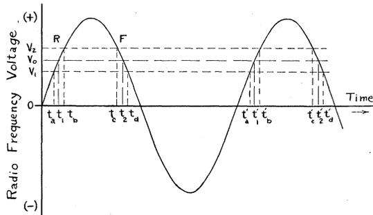
FIG. 3. Voltage-time relations for electron acceleration and deceleration.
