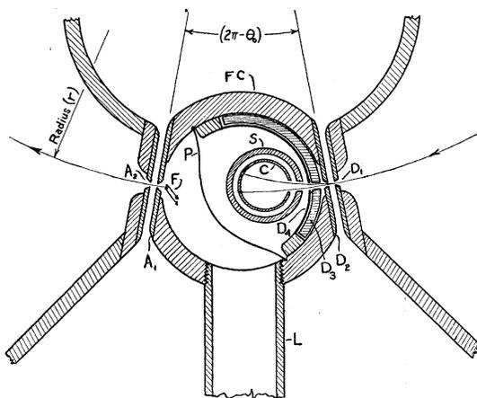
FIG. 2. Cross section of tube in vicinity of filament and collector.
