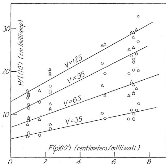
FIG. 7. Deflection per unit current to the cathode  $P/i$  as a function of deflection per unit power input  $F(p)$  for different negative voltages.
