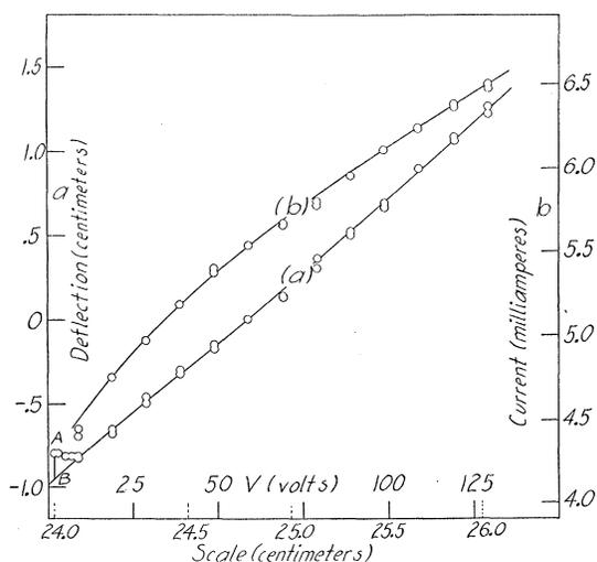
FIG. 3. Deflections and measured currents to the cathode as functions of the negative voltage of the cathode with respect to the surrounding space and of scale readings.
