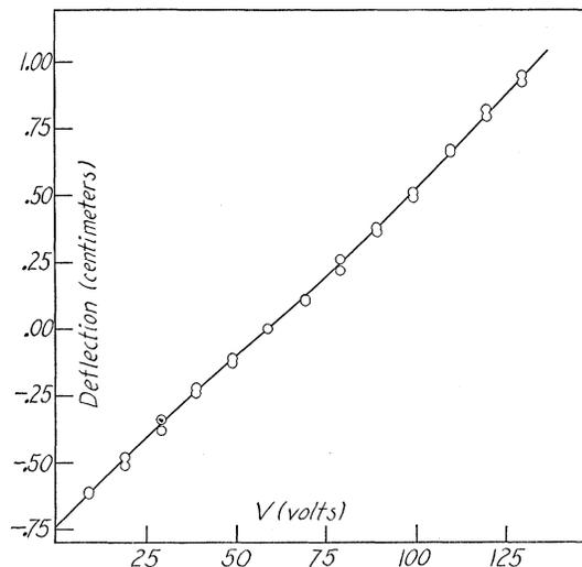
FIG. 4. Deflections resulting from bombardment of the cathode by positive ions as a function of the negative voltage of the cathode with respect to the surrounding space.
