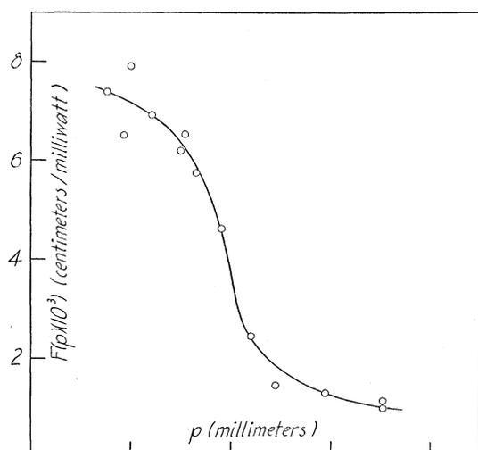
FIG. 6. Deflection per unit power input  $F(p)$  as a function of gas pressure  $p$ .
