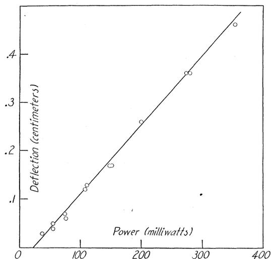
FIG. 5. Deflections resulting from bombardment of the cathode by electrons as a function of electron power input.
