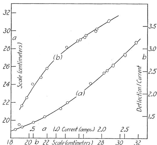
FIG. 2. Curve (a) shows scale readings as a function of arc current when the auxiliary cathode is floating. Curve (b) shows deflection per unit arc current as a function of scale reading.
