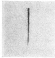
Fig. 2. Double exposures of molybdenum L\alpha_1 line, A, polished face, B, etched face.
