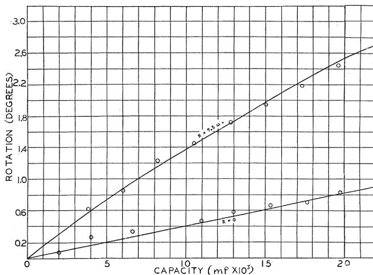
Fig. 4. Rotation-capacity curves.  $L=0.045$  mh;  $R=7.5\omega$  and  $R=0\omega$ . Smooth curves calculated.
