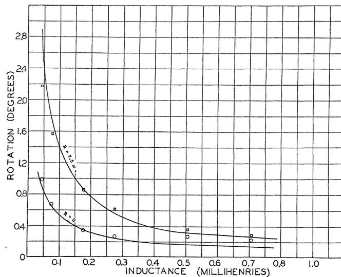
Fig. 5. Rotation-inductance curves.  $C=0.022$  mfd;  $R=7.5\omega$  and  $R=0\omega$ . Smooth curves calculated.
