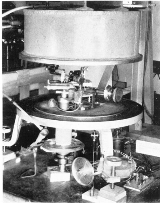
Fig. 3. Photograph of the double-crystal vacuum spectrometer.
