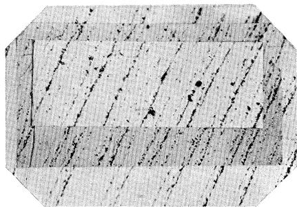
Fig. 12. Superposed photographs of deposits obtained on the same region at different times, the sample being demagnetized after each observation.
