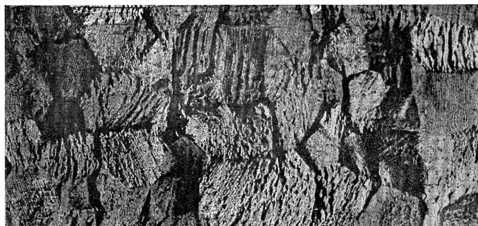
Fig. 1. Deposit on a sample of 4 percent Fe-Si with large grains. Field horizontal. Approximate magnification  $\times 2$ . Deposits are black in all photographs.
