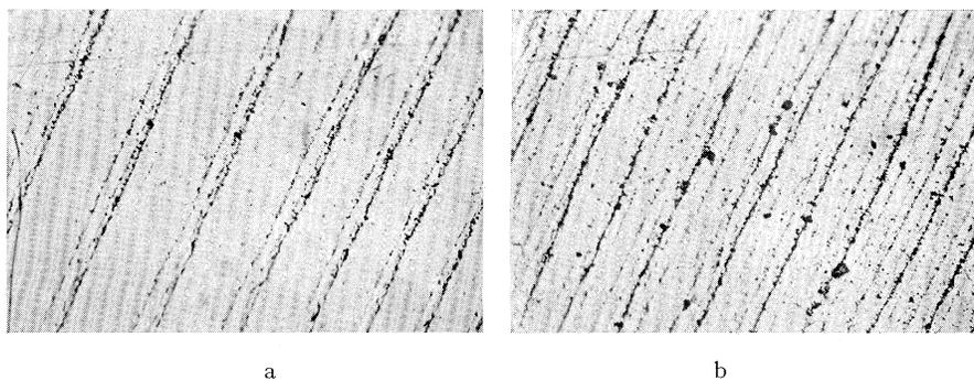
Figs. 11a and 11b. Typical deposits on nickel with the applied field acting in a horizontal direction. Approximate magnification  $\times 65$ .
