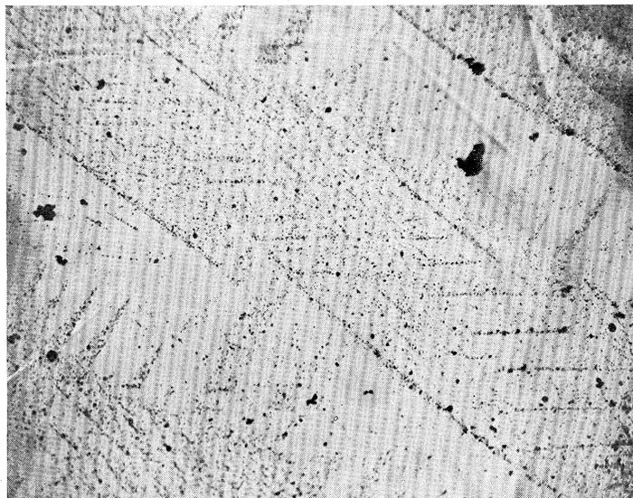
Fig. 10. Deposit on a nickel crystal before magnetization. Approximate magnification  $\times 80$ .
