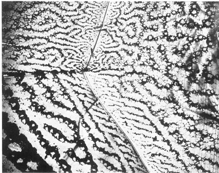
Fig. 7. Deposit on magnetized cobalt near a grain boundary. Approximate magnification  $\times 80$ .
