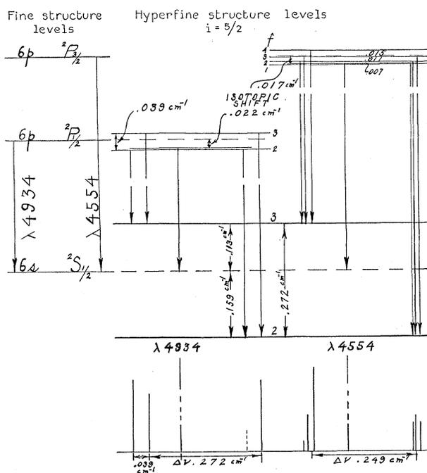
Fig. 1. Hyperfine structure energy level diagram of barium resonance lines, Ba II.
