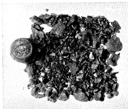
Fig. 2. Piston shattered at 38,000 atmosphere.
