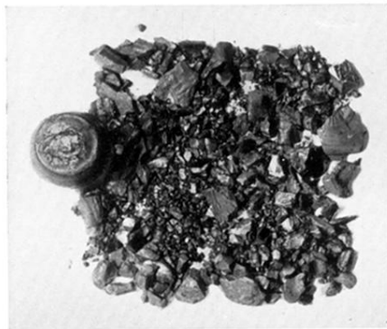
Fig. 2. Piston shattered at 38,000 atmosphere.
