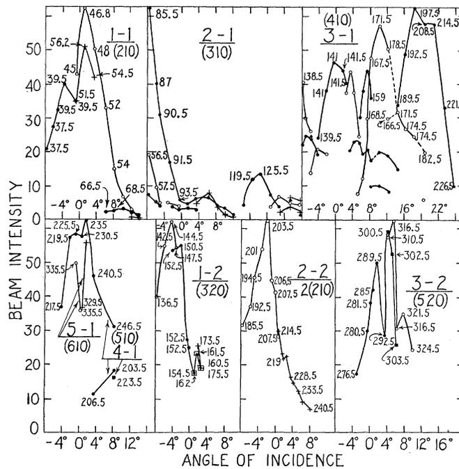
Fig. 9. Curves showing relative intensities of beam components as a function of angle of incidence for the (100) azimuth (uncorrected for background scattering). Plane of reflection is in the (100) azimuth. Designation of beam 3-2 signifies third beam in the second order as per notation in Table I. Values of corrected voltages are given for several of the points.
