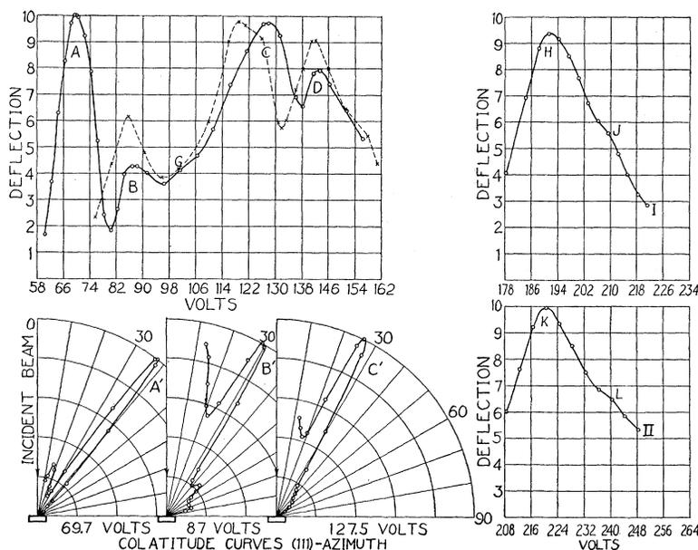
Fig. 3. Curves showing satellites for a copper crystal. The maxima *B* and *D* are the satellites of the main beams *A* and *C*, respectively. *J* and *L* are satellites of *H* and *K*, respectively. The colatitude curves *A'*, *B'*, and *C'* correspond to the maxima *A*, *B*, and *C*, respectively. The dotted curve is for angle of incidence  $-2.5^\circ$ . Curve *I* is for the 3rd beam, 1st order, (100) azimuth; curve *II* for the 4th beam, 1st order, (111) azimuth.
