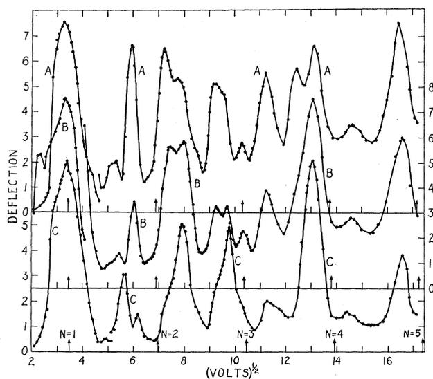
Fig. 5. Regular reflection from the (100) set of planes with the plane of reflection in the (111) azimuth. Curves A, B, and C, are for angles of incidence  $8^\circ$ ,  $10^\circ$ , and  $12^\circ$ , respectively. Arrows indicate positions of theoretical beams for different orders, assuming unit refractive index. Discontinuities in the curves indicate changes in the scale of plotting. Vertical scales which overlap are same for all curves. Zero lines are indicated.
