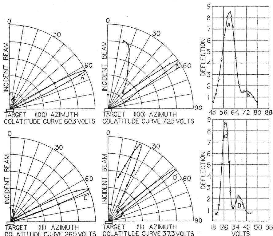
Fig. 2. Curves showing satellites for a copper crystal. The maxima *B* and *D* are the satellites of the main beams *A* and *C*, respectively. The colatitude curves *A'*, *B'*, *C'*, and *D'* correspond to the maxima *A*, *B*, *C*, and *D*, respectively.
