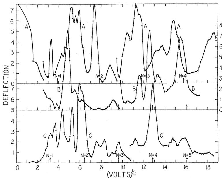
Fig. 13. Regular reflection from the (100) set of planes. Curves *A* and *B* are for angles of incidence of  $40^\circ$  and  $20^\circ$ , respectively, with the plane of reflection in the (100) azimuth. Curve *C* is for angle of incidence  $20^\circ$  with the plane of reflection in the (111) azimuth. Other notation is the same as for Fig. 12.
