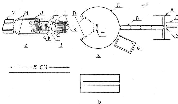
Fig. 1. Apparatus. *a*—top view, *b*—side view of drum, *c*—mounting of crystal, side view, *d*—mounting of crystal, front view.
