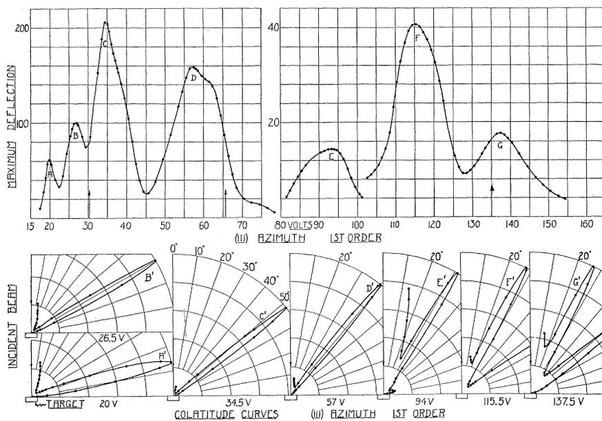
Fig. 6. Curves showing diffraction beams for silver in the 1st order, (111) azimuth below 160 volts for approximately normal incidence. Colatitude curves correspond to maxima in the upper curves which have the same letters.
