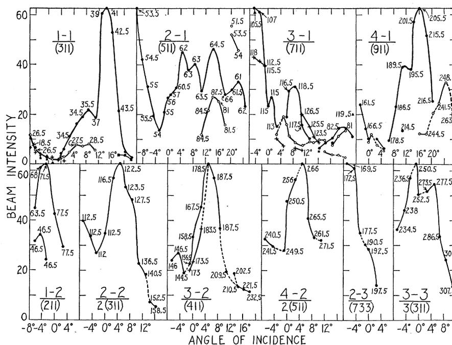
Fig. 10. Curves showing relative intensities of beam components as a function of angle of incidence for the (111) azimuth (uncorrected for background scattering). Plane of reflection is in the (111) azimuth. Notation is the same as in Fig. 9.
