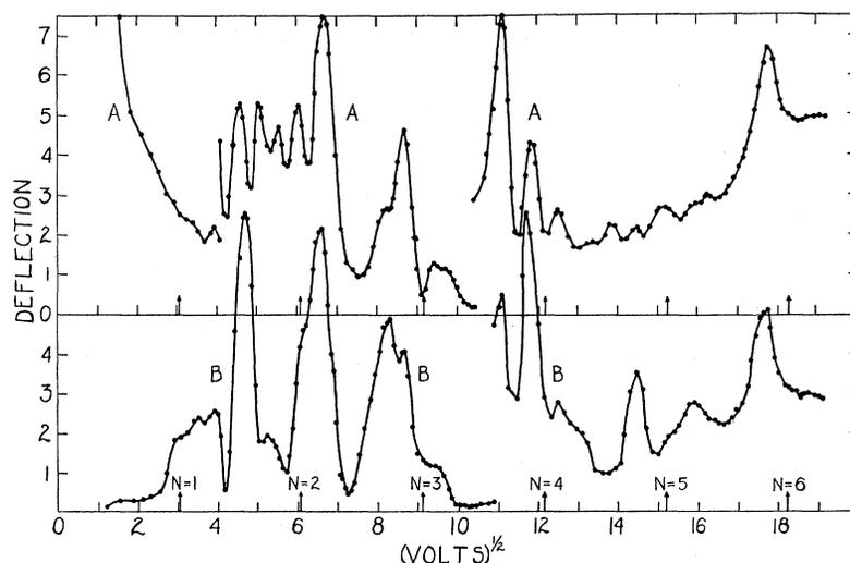
Fig. 12. Regular reflection from the (100) set of planes. Both curves are for angle of incidence  $8.5^\circ$ . For curve A the plane of reflection is in the (100) azimuth. For curve B the plane of reflection is in the (111) azimuth. Arrows indicate positions of theoretical beams for different orders, assuming unit refractive index. Discontinuities in the curves indicate changes in the scale of plotting.
