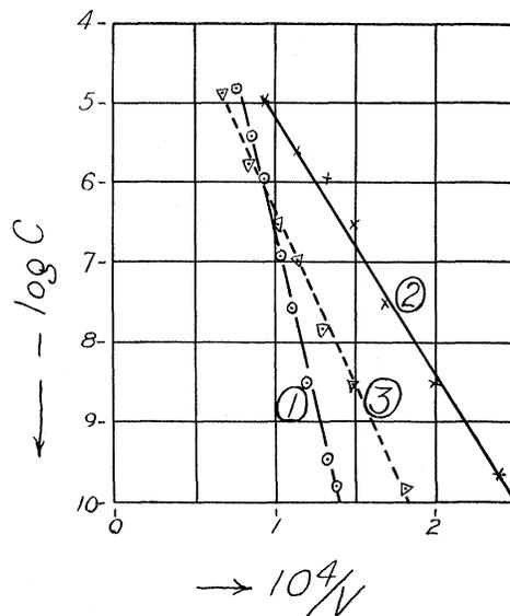
Fig. 6. Field-current characteristics with magnesium anode.
