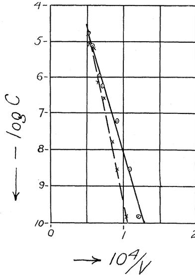
Fig. 4. Field-current characteristics with copper electrodes.
