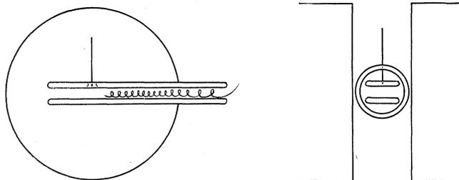
Fig. 1. Arrangement of electrodes in previous experiments.
