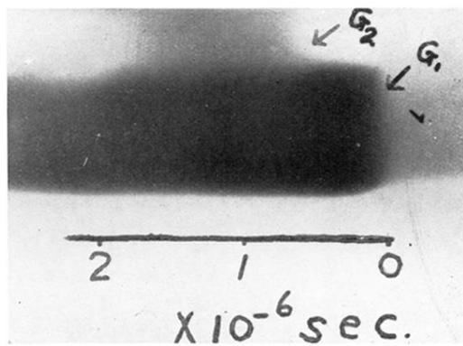
Fig. 2. Photograph of discharge. Electrodes of  $G_2$  brass spheres, 6.5 mm in diameter.
