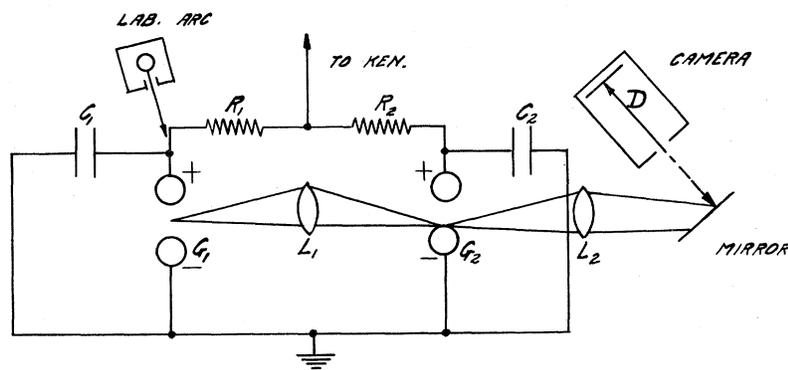
Fig. 1. Diagram of apparatus.  $R_1 = 2.5 \times 10^5$  ohms;  $R_2 = 5 \times 10^5$  ohms;  $C_1 = 0.01$  mfd;  $C_2 = 0.01$  mfd.
