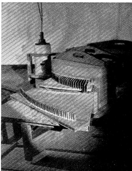
Fig. 5. Photograph showing x-ray tube in cylindrical lead-rubber sheathed housing, scatterer consisting of fifty orientated Ceylon graphite blocks and multicrystal spectrograph with baffles to reduce fogging projecting in front.
