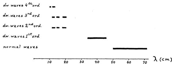
Fig. 11. Regions of the spectrum corresponding to the oscillations generated by vacuum tubes of the type *R5*.
