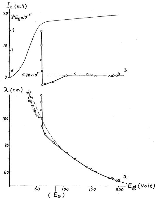
Fig. 9. Curves showing the dependance of the length of the normal waves, the value of the product  $\lambda^2 E_g$  and the emission current on the grid potential. The dotted line (a) corresponds to Barkhausen's Eq. (1).
