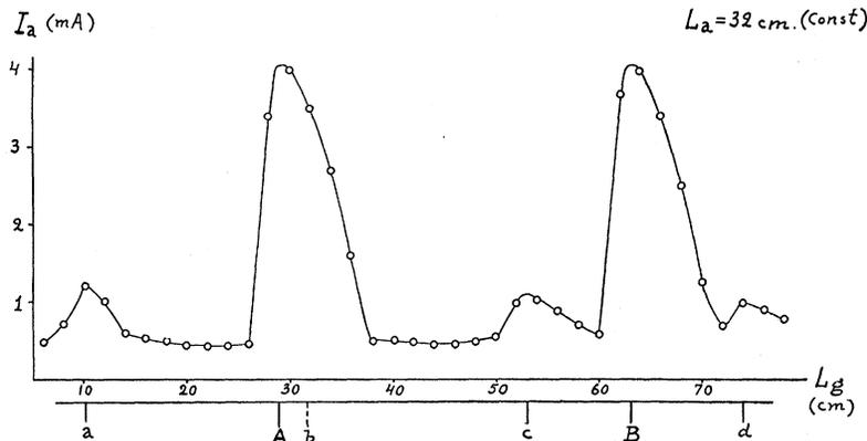
Fig. 4.  $(I_a, L)$ -characteristics, the lengths of the plate circuit and the grid circuit not being equal. The humps A and B correspond to normal waves, humps a, c and d, to dwarf waves.
