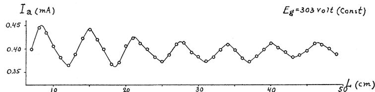
Fig. 8. ( $I_a$ ,  $L$ )-characteristic showing the dependence of the amplitude of oscillations of dwarf waves of the 3<sup>rd</sup> order on the length of the grid and plate circuits.
