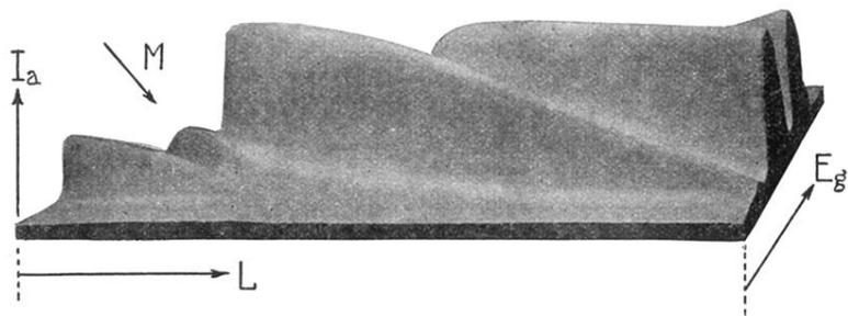
Fig. 2. A 3-dimensional working diagram for vacuum tubes of the type R5.
