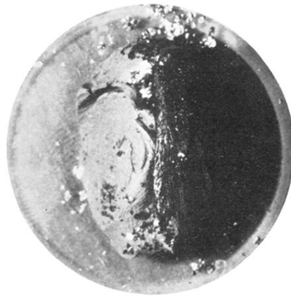
Fig. 3. Photograph of an artificial graphite crystal of approximately natural size. The crystal was broken to show the alignment of the flakes.
