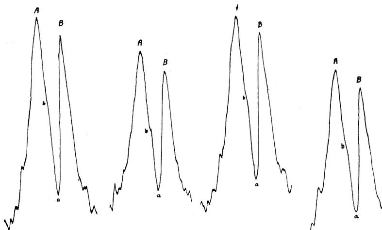
Fig. 3. Microphotometer of absorption of Li 3232Å in lithium vapor. The portion of the trace between *A* and *B* represents the absorption line. It is to be noted that the component *b* is present in each trace and is thereby distinguished from the accidental motions of the galvanometer.
