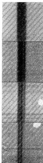
Fig. 1. Absorption of Li 6708 Å in lithium vapor. Temperature of furnace is highest for the top photograph. 6 inch plane grating, dispersion 0.566 Å/mm in fourth order.
