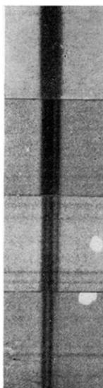
Fig. 1. Absorption of Li 6708A in lithium vapor. Temperature of furnace is highest for the top photograph. 6 inch plane grating, dispersion 0.566 A/mm in fourth order.
