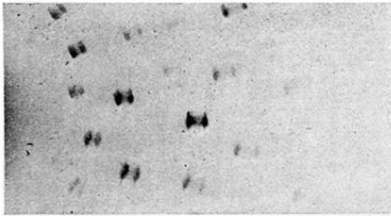
Fig. 1. Laue spots from nonoscillating quartz.
