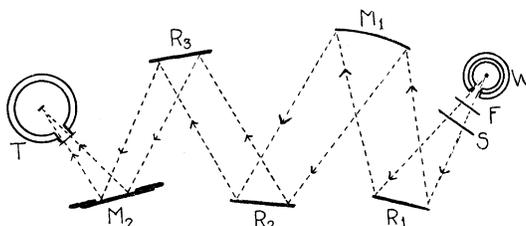
Fig. 1. Reststrahlen apparatus.  $W$ =Welsbach mantel,  $F$ =soot filter,  $R$ =rock-salt plates,  $T$ =microradiometer,  $S$ =glass shutter,  $M$ =silver mirrors.
