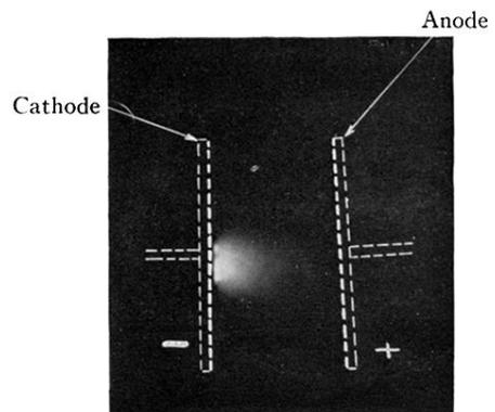
Fig. 2. Low voltage form of 7 amp. D.C. arc between copper plates. The cathode spot moved during the exposure which makes the glow at the cathode surface appear much broader than actually was the case.
