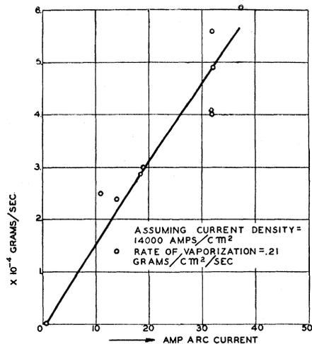
Fig. 6. Vaporization of copper cathode by arc in vacuum.
