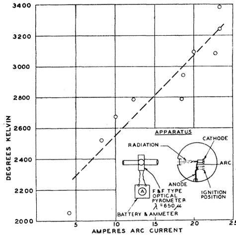
Fig. 5. Apparent temperature—arc current curve. Temperature by optical pyrometer. Emissivity, 0.15.
