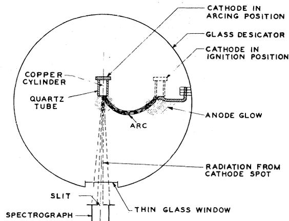
Fig. 3. Arrangement for spectrograms of cathode spot. Cathode was mounted on arm which extended to the outside through flexible bellows.
