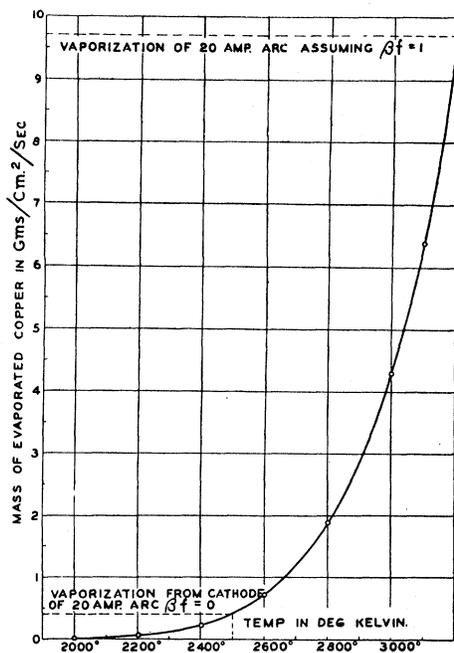
Fig. 7. Rate of vaporization as function of absolute temperature. Plotted from Eq. (22) Phys. Rev. 30, 210, Jones, Langmuir and Mackay.
