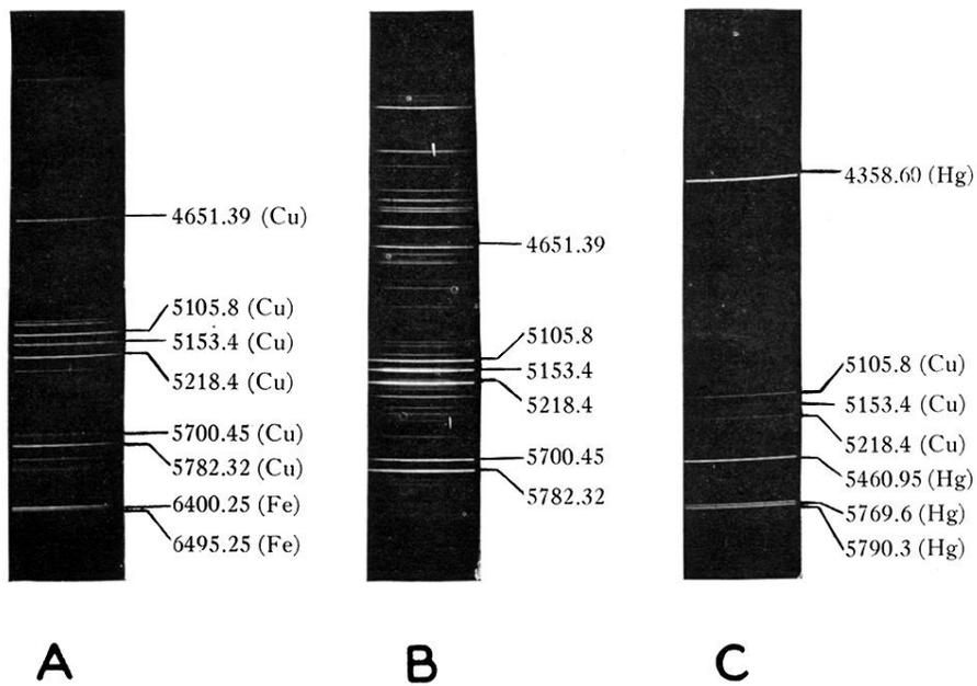
Fig. 4. Spectrograms of vacuum arc. A, cathode spot, vacuum arc between copper electrodes. B, copper arc, atmospheric pressure. C, anode glow, vacuum arc between copper electrodes.
