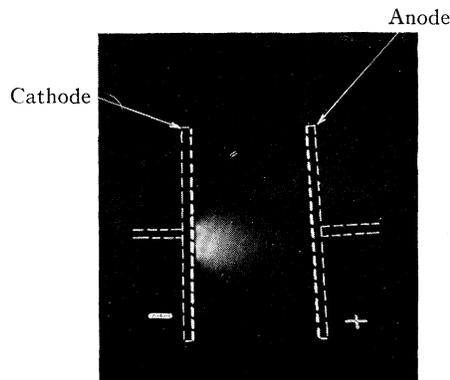
Fig. 2. Low voltage form of 7 amp. D.C. arc between copper plates. The cathode spot moved during the exposure which makes the glow at the cathode surface appear much broader than actually was the case.
