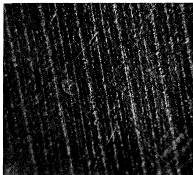
Fig. 5. Pattern obtained on the same grain as that shown in Fig. 4, but at a slightly higher magnetization. Magnification \times 16 .
