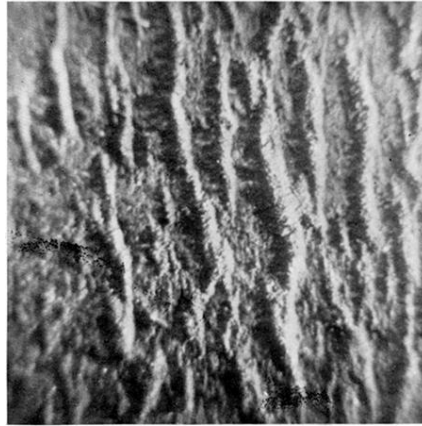
Fig. 1. Patterns obtained on an iron-silicon alloy in large fields. Magnification \times 16 .
