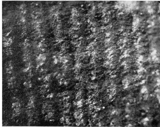
Fig. 2. Pattern obtained on the same sample as that shown in Fig. 1, but at smaller magnetizations. The width of the lines is probably due to surface irregularities. Magnification \times 47 .
