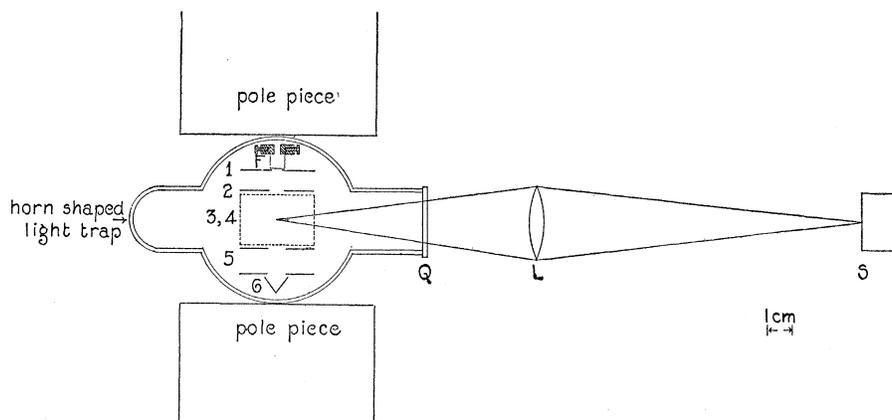
Fig. 2. A cross section showing arrangement of electrodes with respect to the position of the spectrograph.
