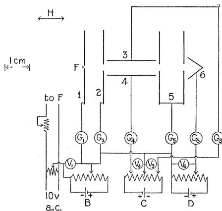
Fig. 1. Arrangement of electrodes and electric circuit.
