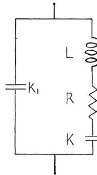
Fig. 5. Equivalent network of piezoelectric plate, and, with modified  $R$  and  $K$ , of plate coupled to fluid column.
