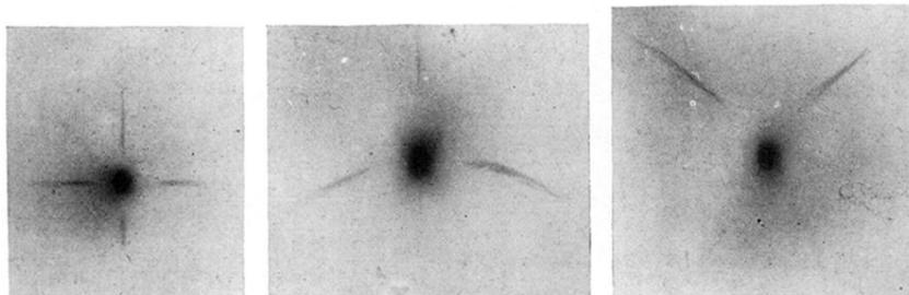
Fig. 5. Diffraction of hydrogen atoms reflected at normal incidence from an LiF crystal.
