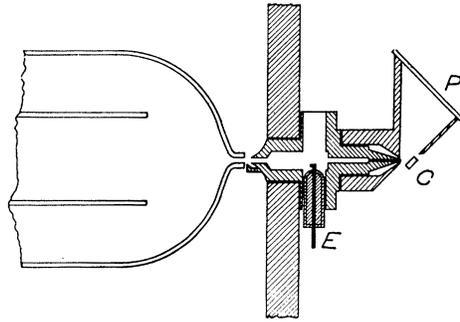
Fig. 8. Arrangement of plate holder for circular patterns.
