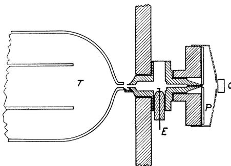
Fig. 1. Collimating system for normal incidence.
