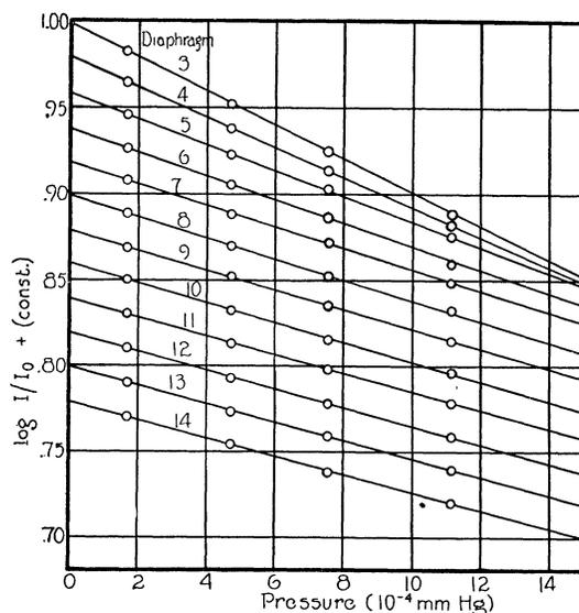
Fig. 2. To show linearity between  $\log I/I_0$  and pressure. (80 volt electrons in mercury vapor.)
