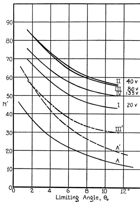
Fig. 5. Number of electrons collected by the scattering chamber, per cm path per primary electron per mm pressure at  $0^\circ\text{C}$ , as a function of the resolving power, in mercury vapor. (Curve A predicted, as the number of primary electrons scattered, by Arnot's results for 80 volt electrons.)
