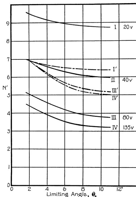
Fig. 6. Number of electrons collected by the scattering chamber, per cm path per primary electron per mm pressure at  $0^\circ\text{C}$ , as a function of the resolving power, in helium.
