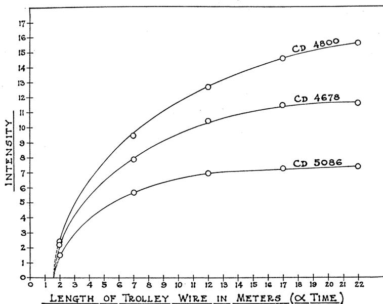
Fig. 4. Intensity of the cadmium arc triplet ( $2^3P_{012} - 2^3S_1$ ).
