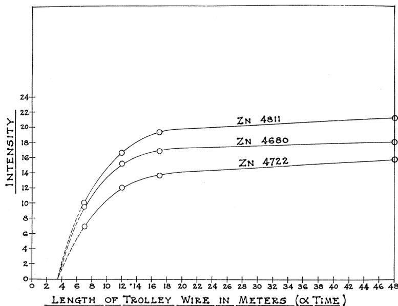
Fig. 2. Intensity of zinc arc triplet ( $2^3P_{012} - 2^3S_1$ ).
