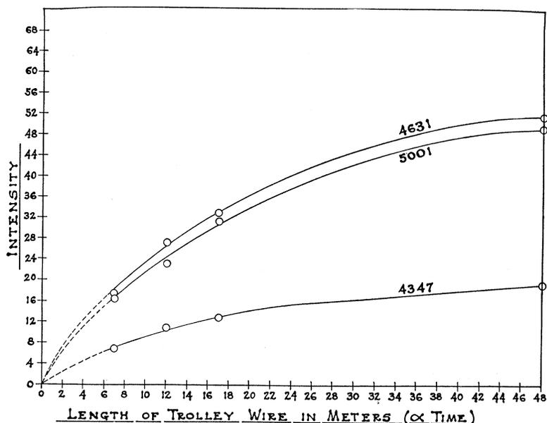
Fig. 3. Intensity of the air lines 5001A, 4631A, and 4347A with zinc spark gap.
