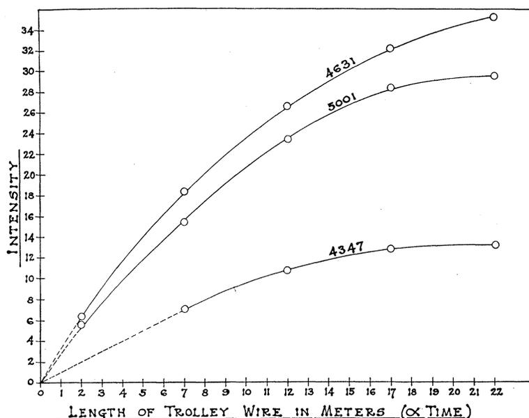
Fig. 5. Intensity of air lines 5001A, 4631A, and 4347A with cadmium spark gap.
