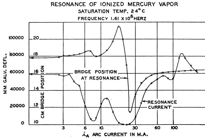
Fig. 5. Resonance characteristic of ionized mercury vapor.
