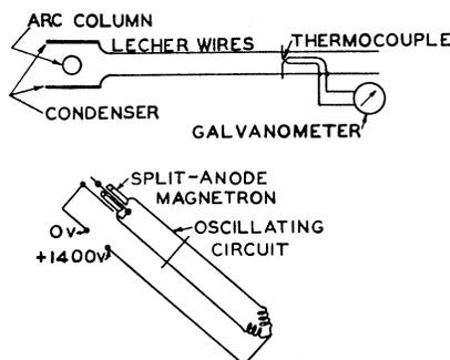
Fig. 4. Apparatus for observing ionized-mercury resonance.
