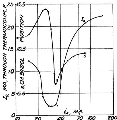
Fig. 13. Resonance characteristic for  $\lambda = 158$  cm.
