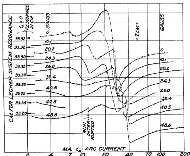
Fig. 15. Effect of transverse magnetic field on plasma-resonance.
