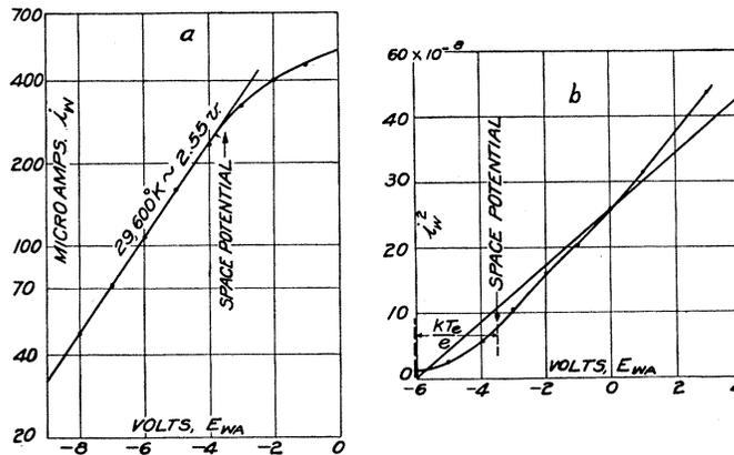
Fig. 6. Electrode volt-ampere characteristics for determining the electron density in the arc.
