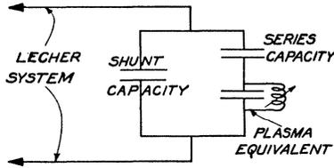
Fig. 2. Qualitative circuit equivalent of a plasma between condenser plates.
