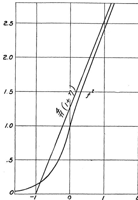
Fig. 7. Theoretical ( $f^2$ ) volt-ampere characteristic and its approximation  $[4(1+\eta)/\pi]$ .
