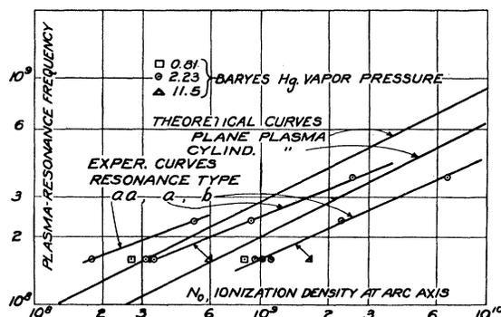
Fig. 9. Comparison of experimental and theoretical plasma-resonance frequencies.
