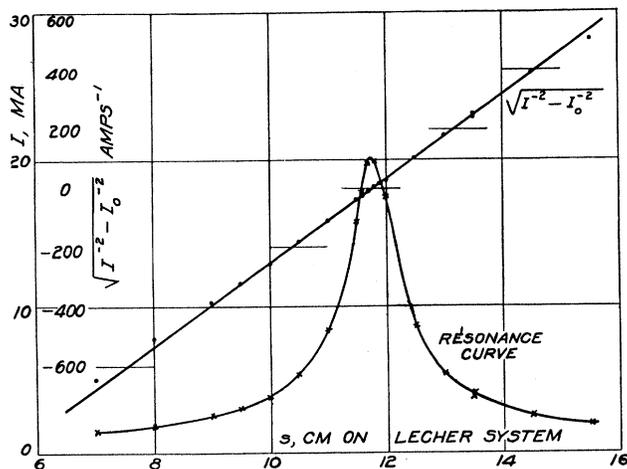
Fig. 12. Lecher system resonance curve and its analysis.
