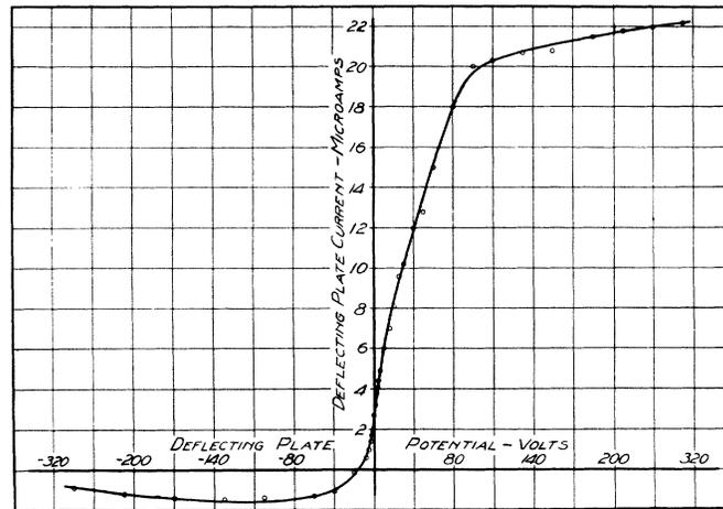
Fig. 3. Plate current for different plate voltages, using deflecting plate *Y*; anode potential 400 volts.
