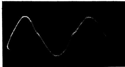
Fig. 4. Effect of non-linearity shown by bump in what should be smooth curve.
