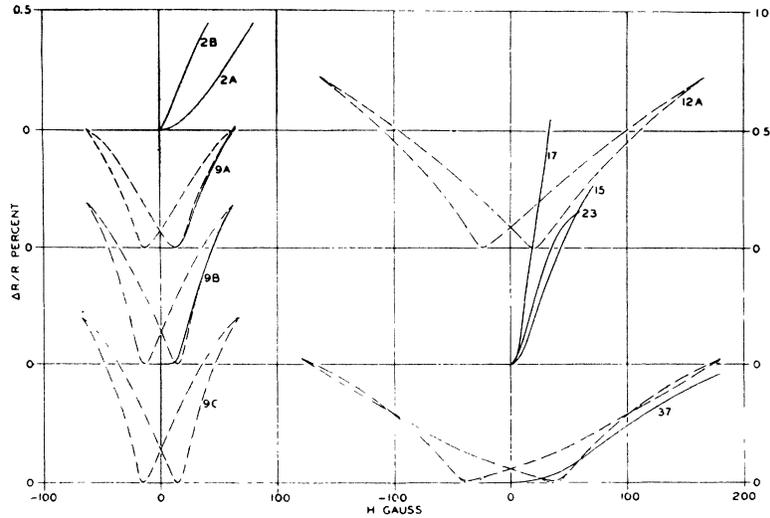
Fig. 1. Longitudinal magneto-resistance in nickel. Previously published results.
