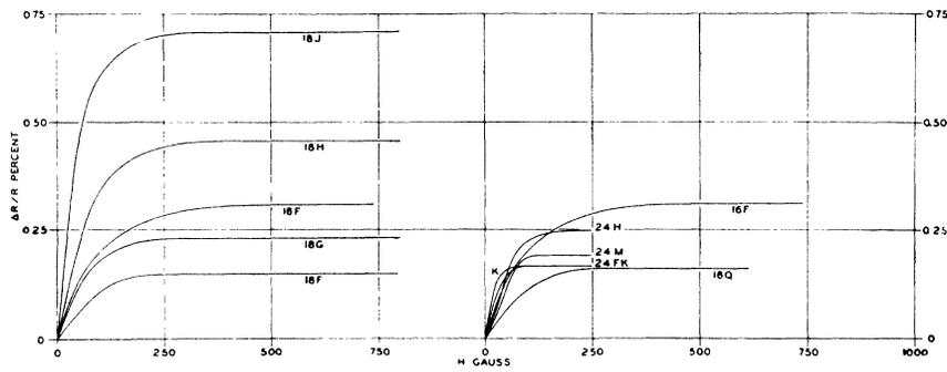
Fig. 4. Longitudinal magneto-resistance in nickel-iron alloys and effect of tension thereon. Previously published results.
