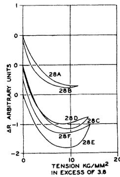
Fig. 6. Elasto-resistance in nickel under tension, after Nobile.
