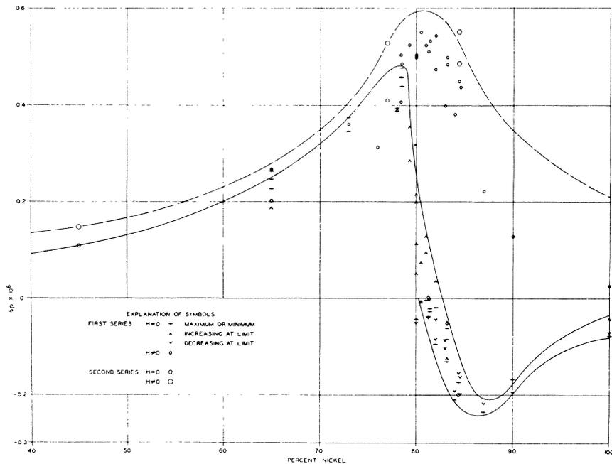
Fig. 10. Magneto-resistance and elasto-resistance in permalloy, as a function of nickel content.
