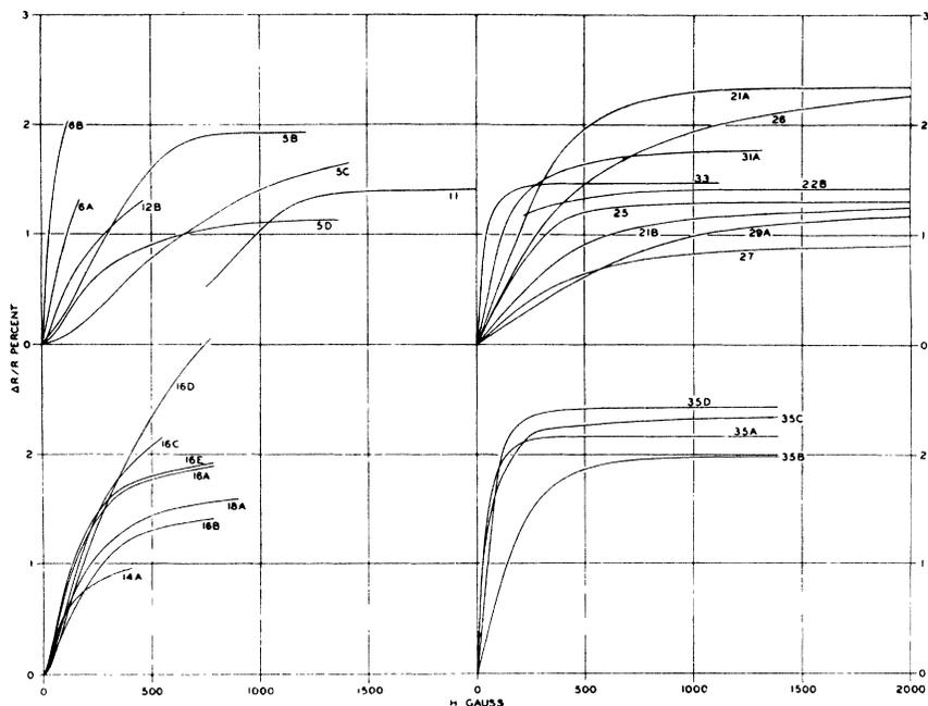
Fig. 2. Longitudinal magneto-resistance in nickel. Presiously published results.
