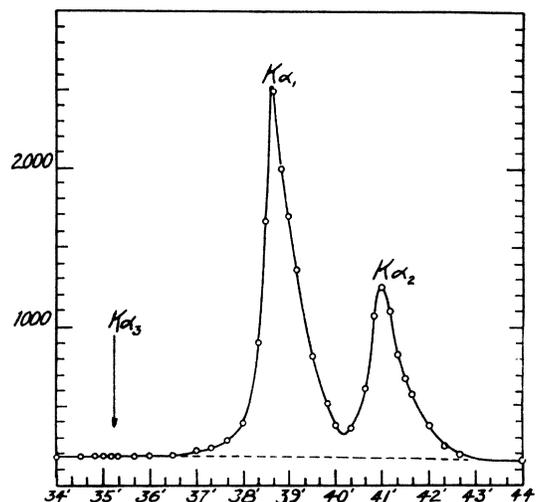
Fig. 1.  $K\alpha_1, \alpha_2$  of copper before taking precautions to reduce background in the neighborhood of  $\alpha_3$ . Note that  $\alpha_3$  is quite imperceptible. The abscissae represent the grazing angles between x-ray beam and calcite crystals.
