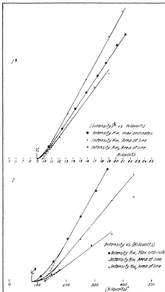
Fig. 5. Intensity of  $K\alpha_1$  and  $K\alpha_3$  as a function of voltage. These curves show how little difference (if any) exists between the excitation voltages of  $\alpha_3$  and  $\alpha_1$ . The upper curve ( $I^{1/3}$  vs k.v.) is plotted for Webster and Clark's relation  $I = \kappa(V - V_0)^{3/2}$  while the lower curve ( $I$  vs. (k.v.)<sup>2</sup>) is plotted for Wooten's relation  $I = C(V^2 - V_0^2)$ .
