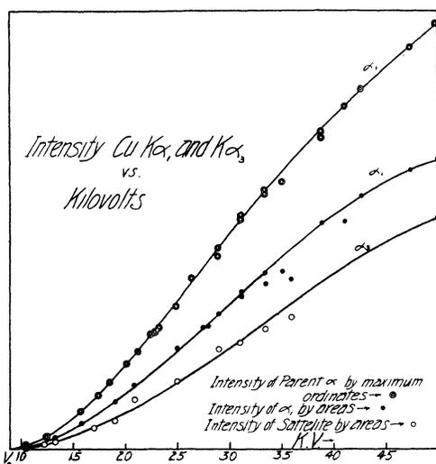
Fig. 7. Intensities of  $K\alpha_3$  and  $K\alpha_1$  for voltages up to five and one half times excitation voltage. method of plotting also leads to the conclusion that  $K\alpha_3$  differs in excitation voltage from  $K\alpha_1$  if at all by less than 200 volts.
