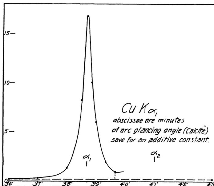
Fig. 2. Typical spectral curve of  $K\alpha_1$  after taking full precautions to reduce background. From such curves as these the areas were taken for the purpose of determining  $\alpha_1$  intensities.
