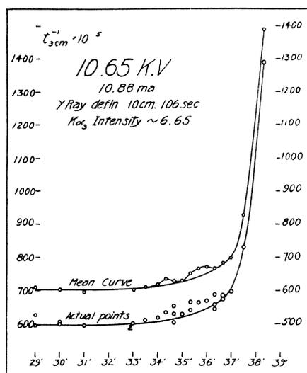
Fig. 4. Spectral curve of  $\text{Cu } K\alpha_3$  at the lowest voltage where it was observed with certainty. Note the doublet structure. The actual observed points as well as the average curve are shown. The voltage here employed differs from the excitation voltage of the  $K$  series of copper by only 1.75 k.v.
