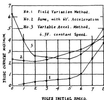
Fig. 3. Efficiency of collection of electrons as a function of their voltage.
