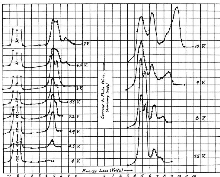
Fig. 4. Energy losses in Hg below ionization.
