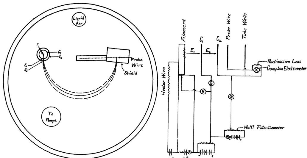
Figs. 1 and 2. Plan of apparatus and electrical circuit.
