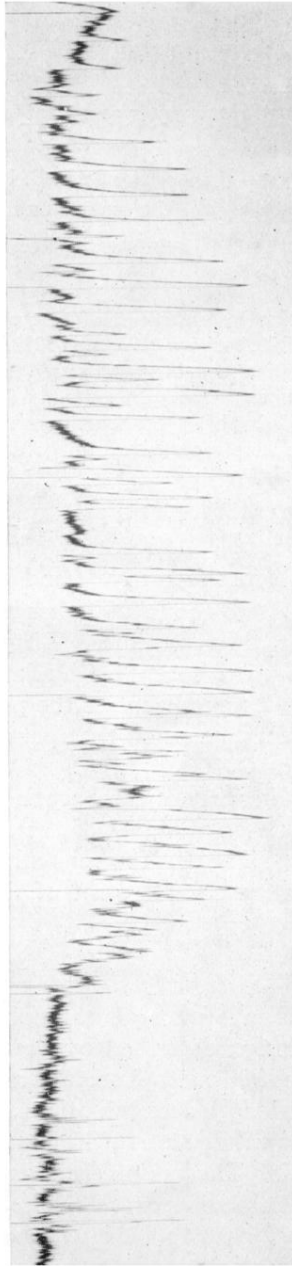
Fig. 2. A microphotometer record of part of the fourth positive band system of CO. from 2090.5A to 1280.6A. Including the hydrogen line 1215.78A, several carbon lines and bands of CO at 1179.3 and 1152.9A.
