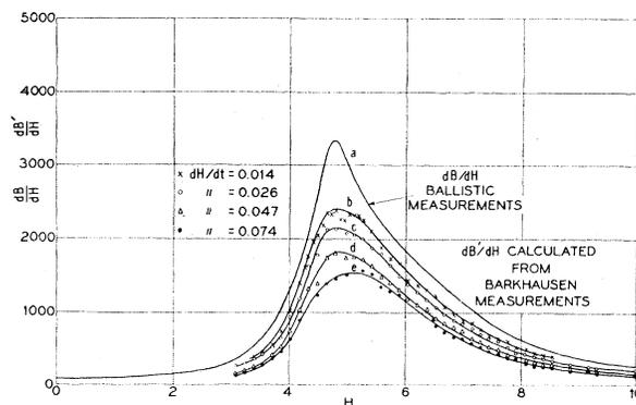
Fig. 4. (a) represents the slope of the lower branch of the hysteresis loop of Fig. 3. The other curves show  $dB/dH$  calculated from Barkhausen measurements using different time rates of change of magnetic field.
