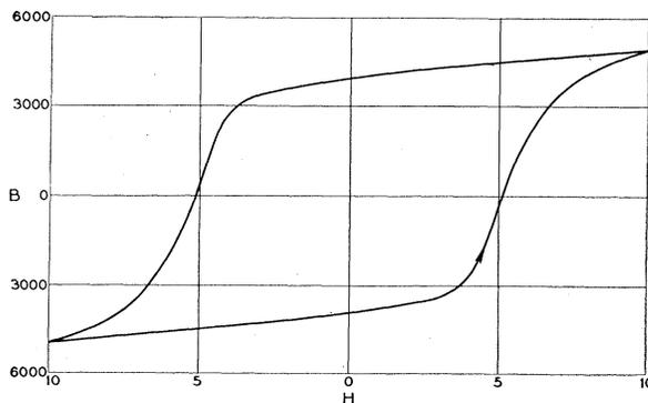
Fig. 3. Hysteresis loop for hard drawn permalloy wire composed of 81 percent Ni and 19 percent Fe.
