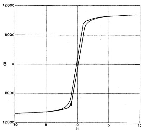
Fig. 6. Hysteresis loop for a sample of annealed permalloy (81 percent Ni, and 19 percent Fe) 1 mm in diameter and 20 cm long.
