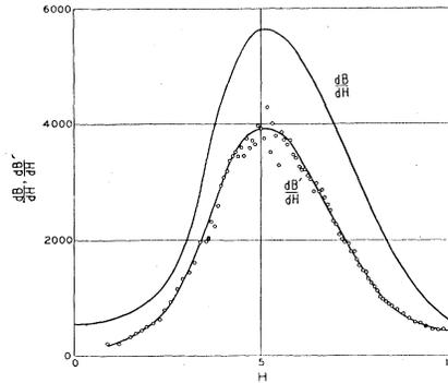
Fig. 11. Barkhausen data for hard drawn iron wire,  $dH/dt=0.011$  gauss/sec.
