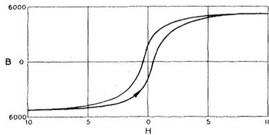
Fig. 14. Hysteresis loop for annealed nickel.
