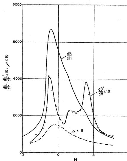
Fig. 9. Barkhausen data for permalloy containing 50 percent Ni and 50 percent Fe,  $dH/dt = 0.046$  gauss/sec.
