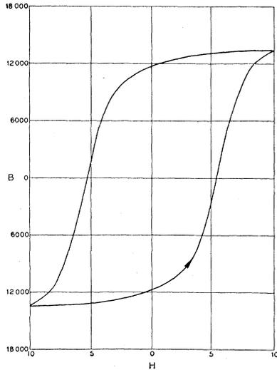
Fig. 10. Hysteresis loop for hard drawn iron wire.
