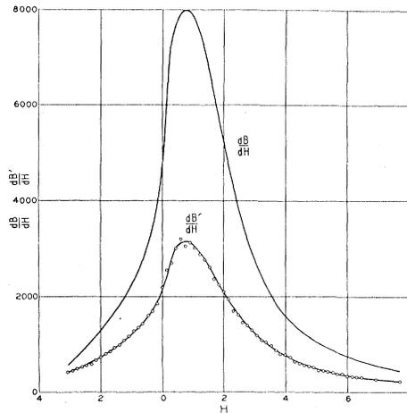
Fig. 13. Barkhausen data for annealed iron,  $dH/dt=0.032$  gauss/sec.
