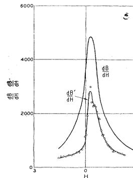
Fig. 15. Barkhausen data for annealed nickel,  $dH/dt = 0.012$  gauss/sec.
