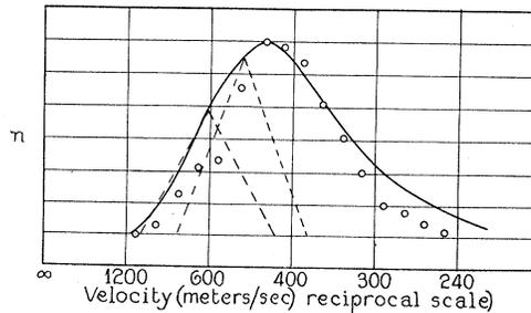
Fig. 5. Comparison of velocity distribution of cadmium atoms before and after reflection.
