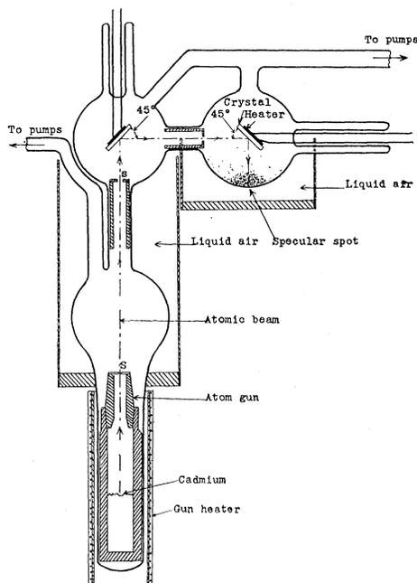
Fig. 1. Type of tube used for successive reflections.
