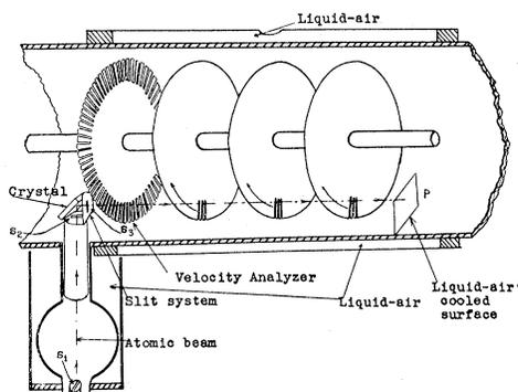
Fig. 3. Apparatus used to measure velocities of reflected atoms.
