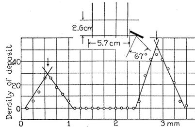
Fig. 4c. Speed of rotor, 76 r.p.s.; velocity of atom beam, 600m/s.
