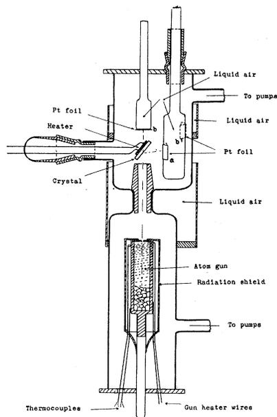
Fig. 6. Type of tube used to obtain quantitative reflection data.
