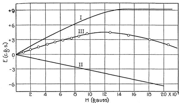
Fig. 7. Resolution of Hall effect into two components for alloy containing 78 percent nickel and 22 percent iron.
