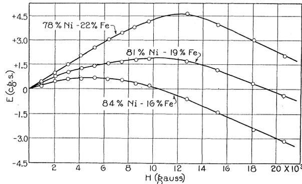
Fig. 4. Comparison of Hall effect in three permalloys of different compositions.
