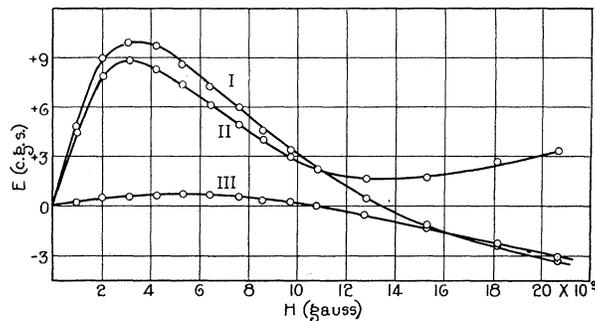
Fig. 1. Hall effect in unannealed permalloy, 84 percent nickel and 16 percent iron; Curve I for magnetic field in one direction; Curve II for magnetic field in opposite direction; Curve III algebraic mean of Curve I and Curve II.
