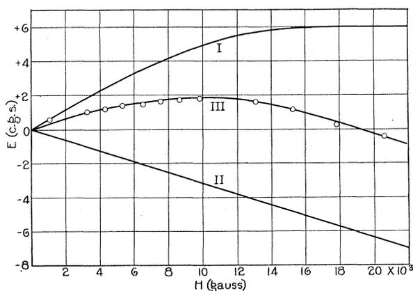
Fig. 6. Resolution of Hall effect into two components for alloy containing 81 percent nickel and 19 percent iron.
