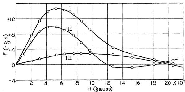
Fig. 2. Hall effect in unannealed permalloy, 81 percent nickel and 19 percent iron; Curve I for magnetic field in one direction; Curve II for magnetic field in opposite direction; Curve III algebraic mean of Curve I and Curve II.
