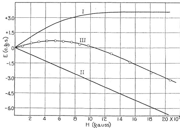
Fig. 5. Resolution of Hall effect into two components for alloy containing 84 percent nickel and 16 percent iron.
