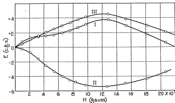
Fig. 3. Hall effect in unannealed permalloy, 78 percent nickel and 22 percent iron; Curve I for magnetic field in one direction; Curve II for magnetic field in opposite direction; Curve III algebraic mean of Curve I and Curve II.
