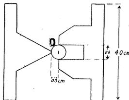
Fig. 2. Diagrammatic sketch of pole pieces (cross-section).
