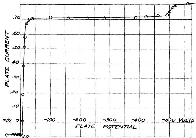
Fig. 4. Total plate current as a function of plate voltage with the grid at  $-500$  volts. Positive ordinates indicate an excess of positive ions to the plate, negative ordinates indicate an electron current from grid to the plate.
