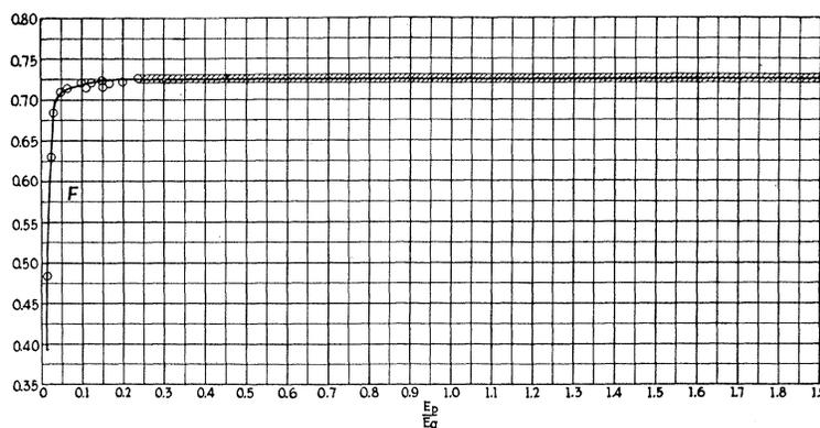
Fig. 6. Curve showing the fraction,  $F$ , of the total positive ion emission that reaches the plate as a function of the ratio  $E_p/E_g$ .
