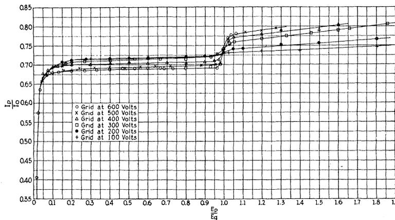
Fig. 5. Curves showing the ratio of the plate current,  $I_p$ , to the emission current,  $I_0$ , as a function of the ratio of the plate potential,  $E_p$ , to the grid potential,  $E_g$ .
