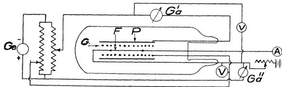
Fig. 1. Diagram of tube and electrical connections.
