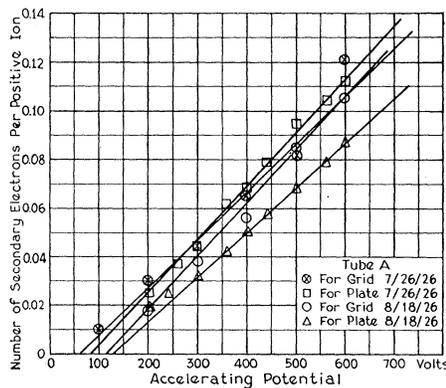
Fig. 3. Secondary electron emission produced at the grid and plate by caesium positive ions. Tube A.
