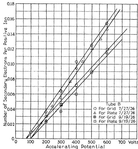
Fig. 2. Secondary electron emission produced at the grid and plate by caesium positive ions. Tube B.
