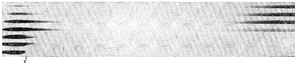
Fig. 3. Taken with the same spectrograph as Fig. 2, but with a neocyanine plate. Temperature and density increasing downward. E indicates infra-red edge. Comparison spectrum neon.
