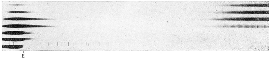
Fig. 3. Taken with the same spectrograph as Fig. 2, but with a neocyanine plate. Temperature and density increasing downward. E indicates infra-red edge. Comparison spectrum neon.
