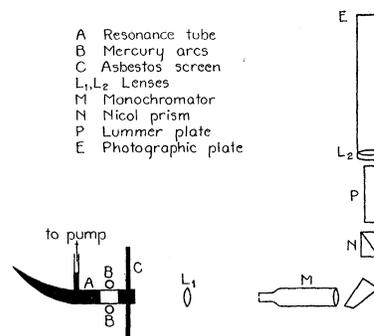
Fig. 1. Arrangement of apparatus.
