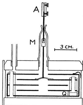
Fig. 2. Design of the test condenser.
