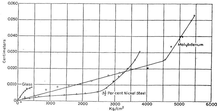
Fig. 4. Curves of sideways deflection at end of shaft plotted against downward deflection and maximum stress intensity.
