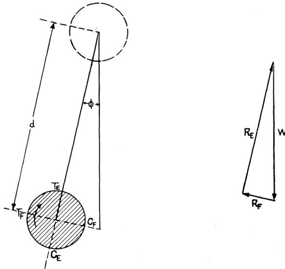
Fig. 3. View of weighted end of shaft showing sideways deflection due to internal friction.
