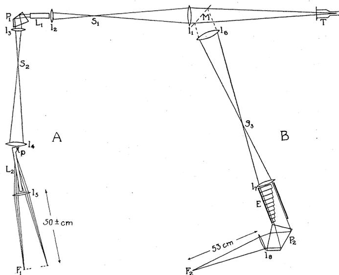
Fig. 1. Arrangement of spectroscopes. *T*, vacuum tube; *M*, plane mirror; *l*<sub>1</sub> ··· *l*<sub>8</sub>, lenses; *L*<sub>1</sub>, *L*<sub>2</sub>, small and large Lummer plates; *P*<sub>1</sub>, *P*<sub>2</sub>, prisms; *F*<sub>1</sub>, *F*<sub>2</sub>, focal planes of *l*<sub>5</sub> and *l*<sub>8</sub>; *S*<sub>1</sub>, *S*<sub>2</sub>, *S*<sub>3</sub>, slits; *p*, rotation point of large plate.
