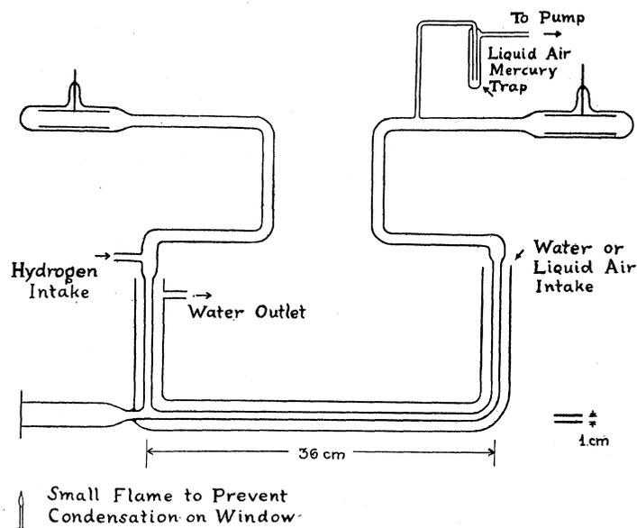
Fig. 2. Vacuum tube used as source.
