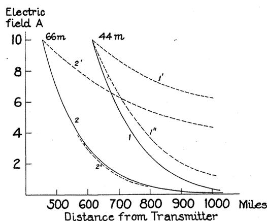
Fig. 3. The electric field as a function of the distance from the transmitter for a 44 and a 66 meter wave; curves 1 and 2 observed, curves 1' and 2' calculated by the inverse distance law, curves 1'' and 2'' calculated from (15).
