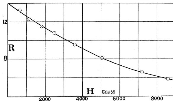
Fig. 1. Variation of the Hall coefficient,  $R$ , with the field strength,  $H$ .
